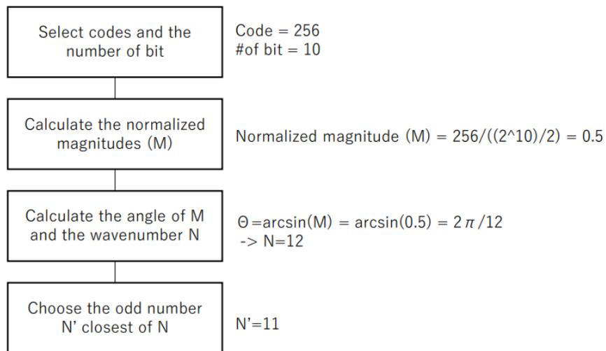
Fig. 3.13 Flowchart of  $\omega_2$  in  $f_{11}(t)$
