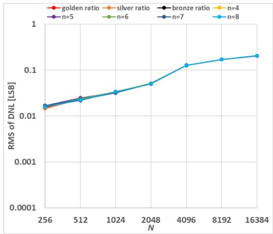
Fig. 4.4 Resolution characteristics of RMS of DNL of metallic ratio samplings
