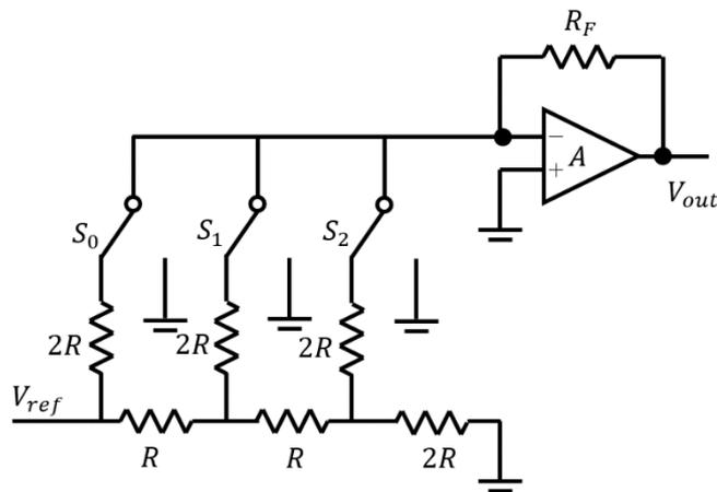
Fig. 2.11 3-bit Current switching type structure
