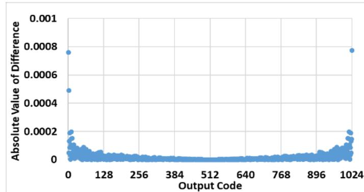
Fig. 3.6 Absolute value of the difference between DNLs calculated from the method in Section 3.3 and the ideal histogram.
