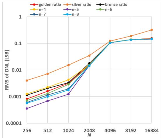
Fig. 4.1 Resolution characteristics of RMS of DNL of metallic ratio samplings
