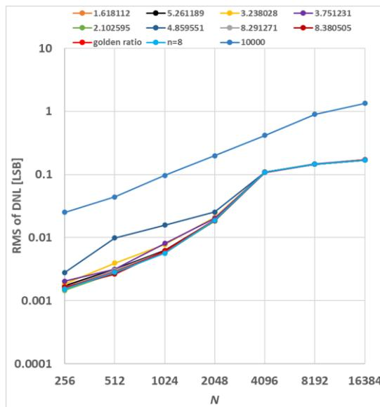
Fig. 4.18 Comparison of resolution characteristics of RMS of DNL of metallic ratio samplings with those of real number ratio sampling (noise 0.001%)
