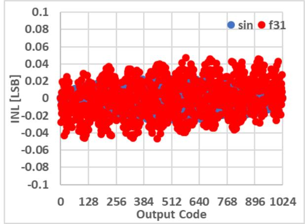
Fig. 3.22 Ideal 10-bit ADC INL for the input signal of  $f_{31}(t) = 1.2 \left( \sin(t) - \frac{\sin(31t)}{50} \right)$  in red and  $f(t) = \sin(t)$  in blue
