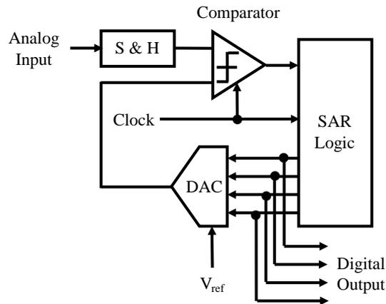
Fig. 3.1 Block diagram of typical SAR ADC
