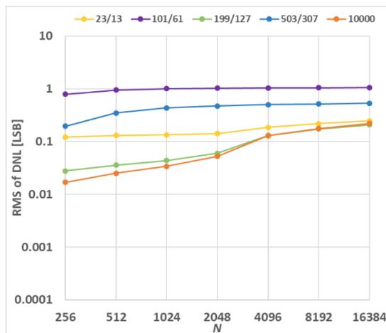
Fig. 4.8 Resolution characteristics of RMS of DNL of prime number ratio samplings by a pair of relatively smaller prime numbers (noise 0.1%)
