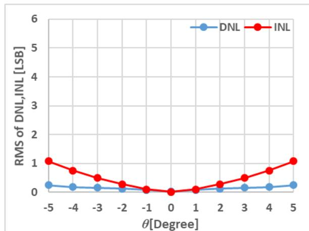
Fig. 3.28 Phase error characteristics of RMS of DNL, INL
