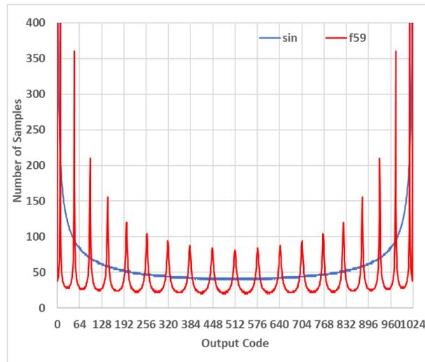
Fig. 3.20 Ideal 10-bit ADC output histogram for the input signal of  $f_{59}(t) =$
