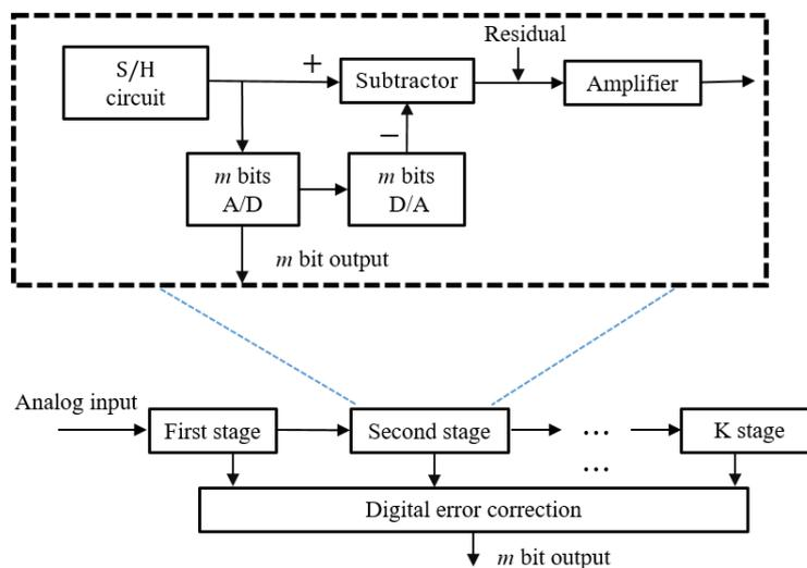
Fig. 2.7 Pipeline ADC structure block diagram.
