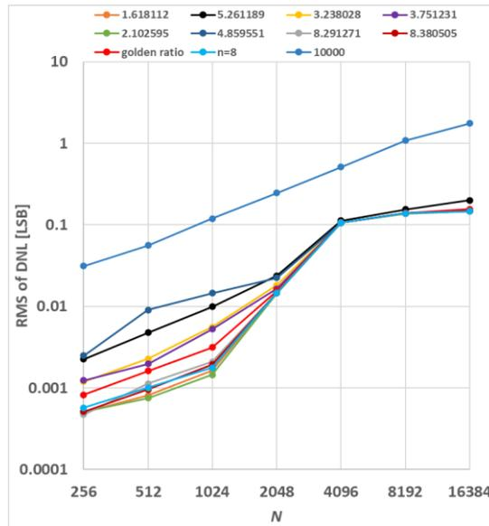
Fig. 4.17 Comparison of resolution characteristics of RMS of DNL of metallic ratio samplings with those of real number ratio sampling (no noise)
