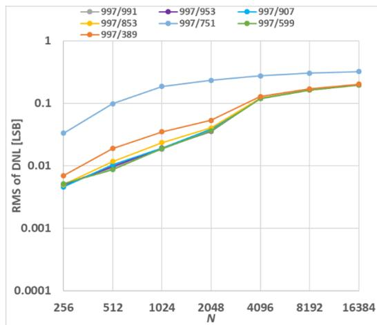
Fig. 4.11 Resolution characteristics of RMS of DNL of prime number ratio samplings by a pair of relatively larger prime numbers (noise 0.01%)
