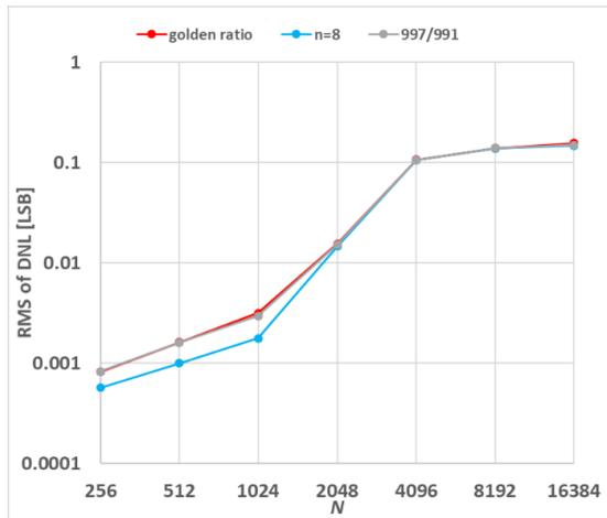
Fig. 4.13 Comparison of resolution characteristics of RMS of DNL of metallic ratio samplings with those of prime number ratio sampling (no noise)
