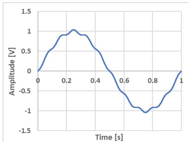
Fig. 3.15 Input wave  $f_{11}(t) = \sin(t) - \frac{\sin(11t)}{25}$
