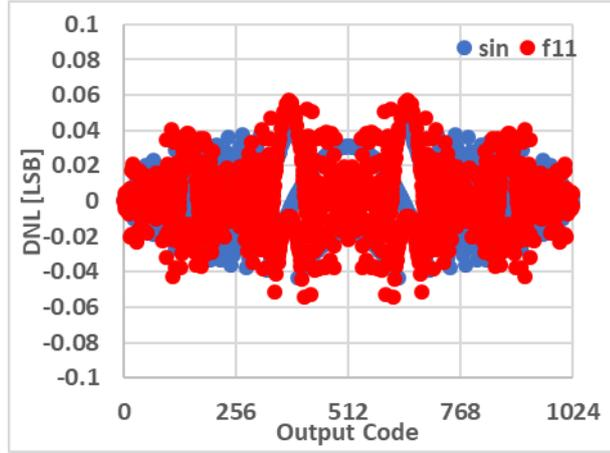
Fig. 3.17 Ideal 10-bit ADC DNL for the input signal of  $f_{11}(t) = \sin(t) - \frac{\sin(11t)}{25}$  in red and  $f(t) = \sin(t)$  in blue
