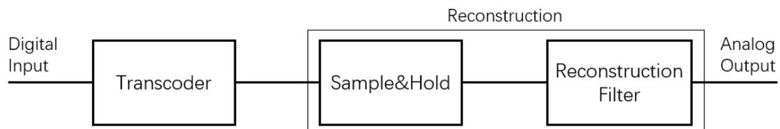
Fig. 2.2 Block diagram of the basic functions of a DAC.
