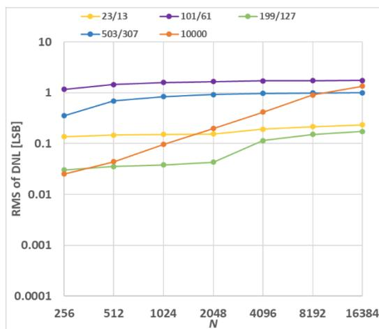
Fig. 4.6 Resolution characteristics of RMS of DNL of prime number ratio samplings by a pair of relatively smaller prime numbers (noise 0.001%)
