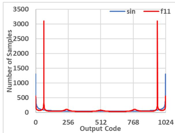
Fig. 3.16 Ideal 10-bit ADC output histogram for the input signal of  $f_{11}(t) =$
