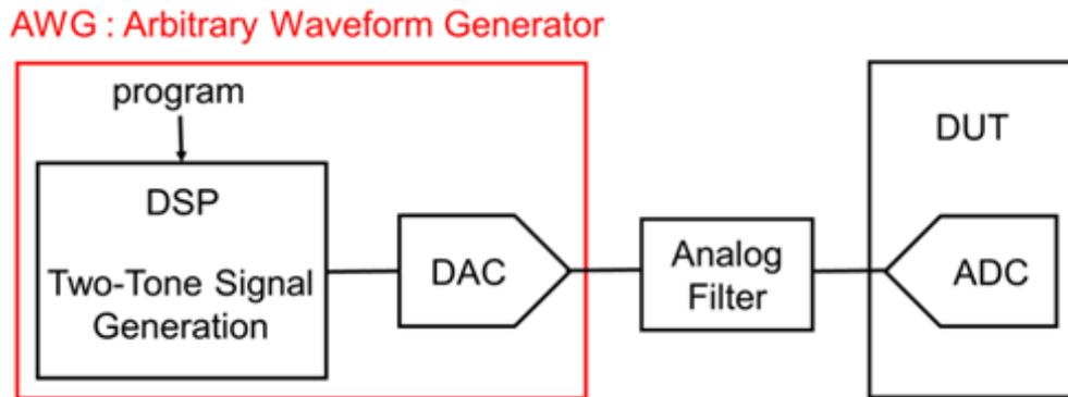
Fig. 3.7 Hardware components for generating proposed two-tone sine wave
