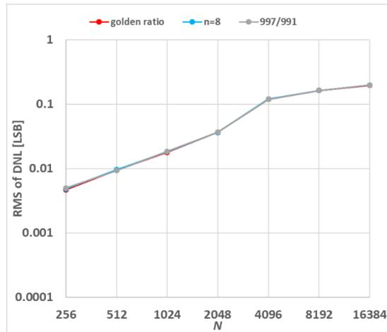
Fig. 4.15 Comparison of resolution characteristics of RMS of DNL of metallic ratio samplings with those of prime number ratio sampling (noise 0.01%)
