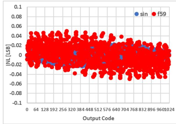
Fig. 3.24 Ideal 10-bit ADC INL for the input signal of  $f_{59}(t) = 1.2 \left( \sin(t) - \frac{\sin(59t)}{100} \right)$  in red and  $f(t) = \sin(t)$  in blue
