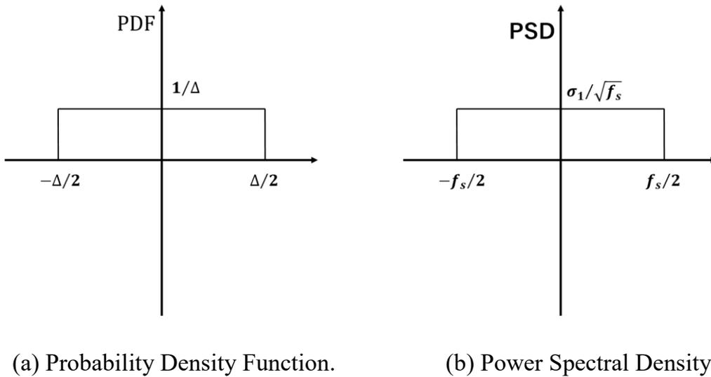
Fig. 2.4 Quantization noise.
