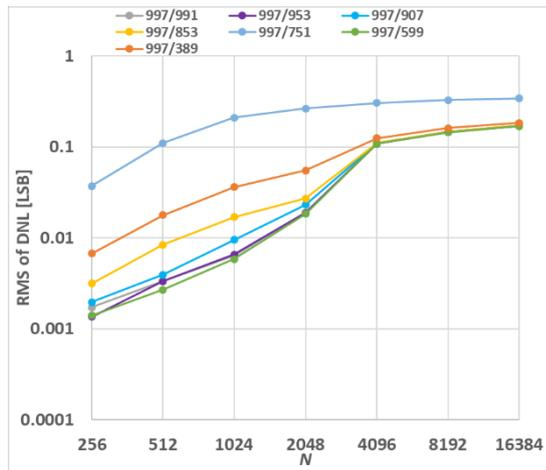
Fig. 4.10 Resolution characteristics of RMS of DNL of prime number ratio samplings by a pair of relatively larger prime numbers (noise 0.001%)
