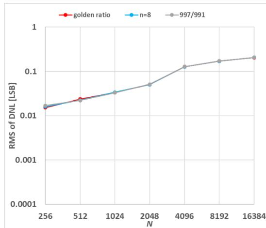
Fig. 4.16 Comparison of resolution characteristics of RMS of DNL of metallic ratio samplings with those of prime number ratio sampling (noise 0.1%)
