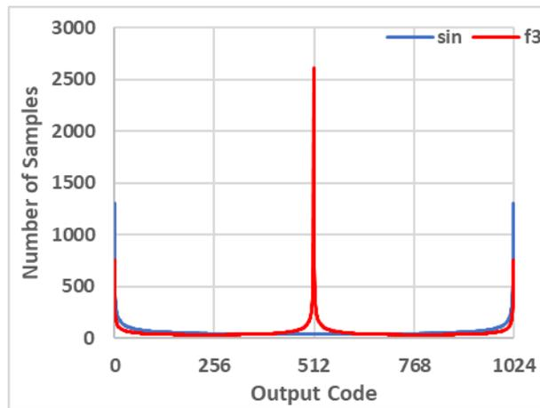
Fig. 3.10 Ideal 10-bit ADC output histogram for the input signal of  $f_3(t) =$
