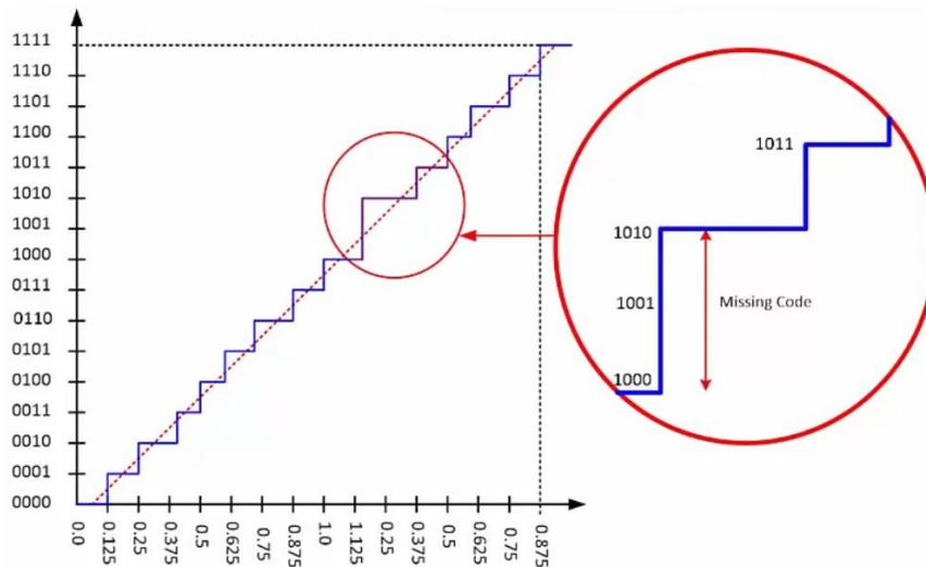
Fig. 2.15 Missing code
