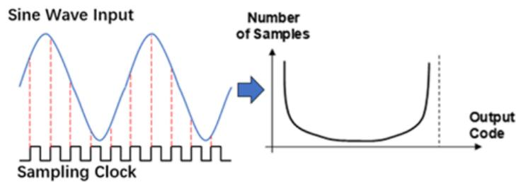
Fig. 3.3 Histogram generation for sine wave input
