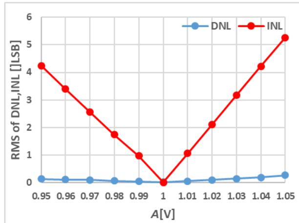
Fig. 3.27 Amplitude error characteristics of RMS of DNL, INL
