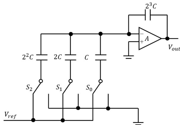
Fig. 2.12 3-bit Capacity switching type structure
