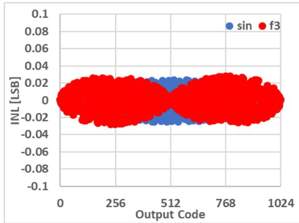
Fig. 3.12 Ideal 10-bit ADC INL for the input signal of  $f_3(t) = \sin(t) - \frac{\sin(3t)}{3}$  in red and  $f(t) = \sin(t)$  in blue
