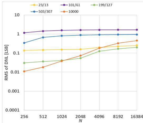
Fig. 4.7 Resolution characteristics of RMS of DNL of prime number ratio samplings by a pair of relatively smaller prime numbers (noise 0.01%)
