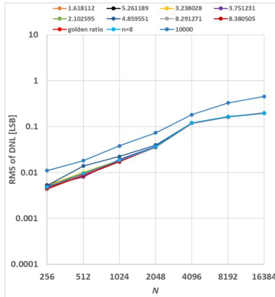
Fig. 4.19 Comparison of resolution characteristics of RMS of DNL of metallic ratio samplings with those of real number ratio sampling (noise 0.01%)
