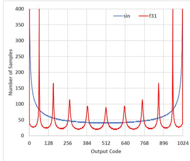
Fig. 3.19 Ideal 10-bit ADC output histogram for the input signal of  $f_{31}(t) =$
