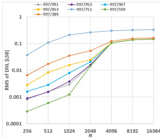
Fig. 4.9 Resolution characteristics of RMS of DNL of prime number ratio samplings by a pair of relatively larger prime numbers (no noise)
