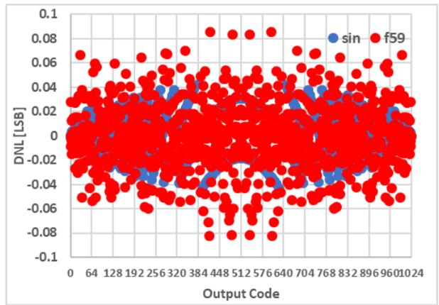
Fig. 3.23 Ideal 10-bit ADC DNL for the input signal of  $f_{59}(t) = 1.2 \left( \sin(t) - \frac{\sin(59t)}{100} \right)$  in red and  $f(t) = \sin(t)$  in blue
