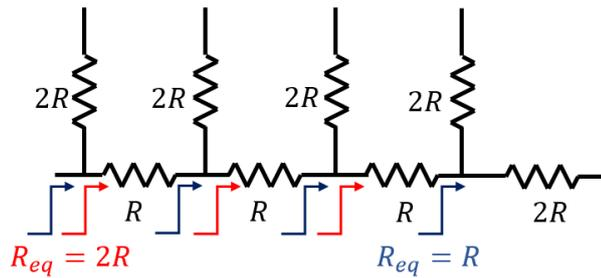
Fig. 2.10 R-2R ladder structure
