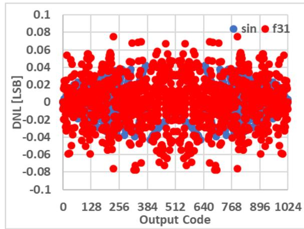
Fig. 3.21 Ideal 10-bit ADC DNL for the input signal of  $f_{31}(t) = 1.2 \left( \sin(t) - \frac{\sin(31t)}{50} \right)$  in red and  $f(t) = \sin(t)$  in blue
