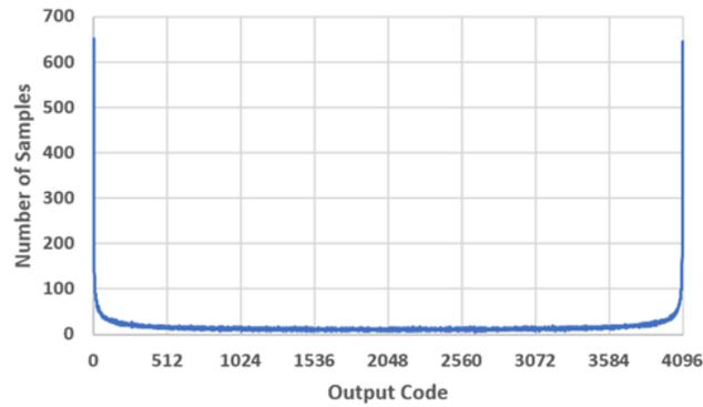
Fig. 3.4 Ideal 12-bit ADC output histogram for the sine wave input
