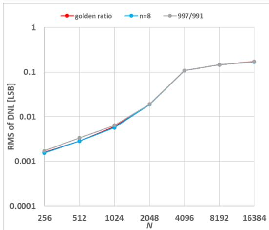
Fig. 4.14 Comparison of resolution characteristics of RMS of DNL of metallic ratio samplings with those of prime number ratio sampling (noise 0.001%)
