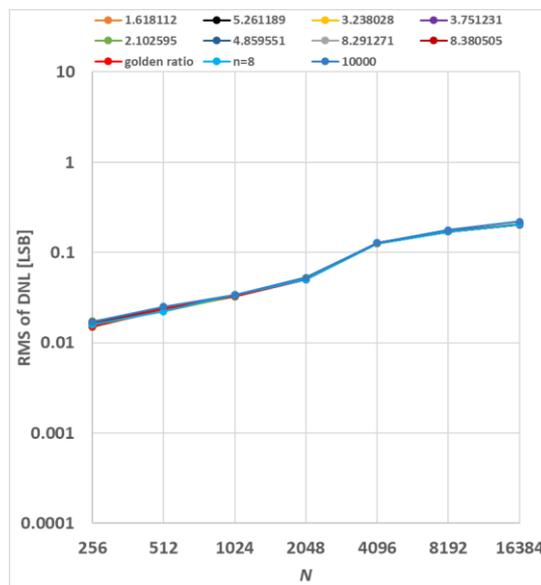
Fig. 4.20 Comparison of resolution characteristics of RMS of DNL of metallic ratio samplings with those of real number ratio sampling (noise 0.1%)
