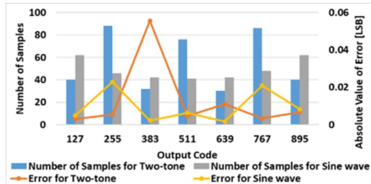
Fig. 3.25 Comparison of ideal ADC using sine wave and two-tone input ( $f_{11}(t)$ ) histograms.
