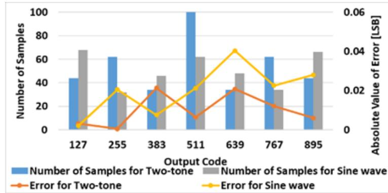
Fig. 3.26 Comparison of obtained DNL errors of non-ideal ADC using sine wave and two-tone input ( $f_{11}(t)$ ) histograms.
