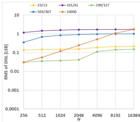
Fig. 4.5 Resolution characteristics of RMS of DNL of prime number ratio samplings by a pair of relatively smaller prime numbers (no noise)
