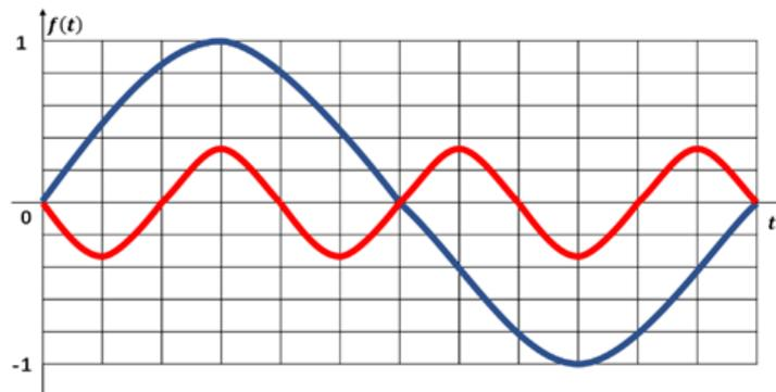
Fig. 3.8 Waveforms  $f(t) = \sin(t)$  in blue and  $f(t) = -\frac{\sin(3t)}{3}$  in red
