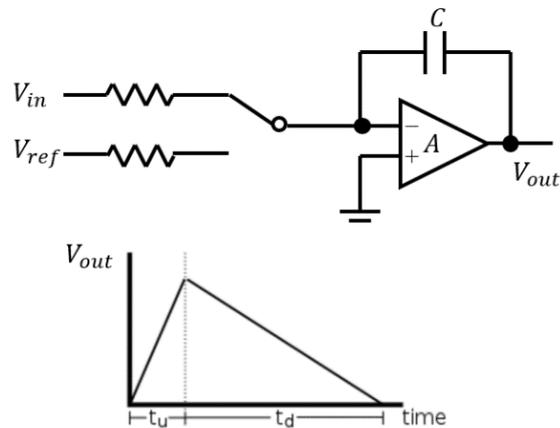
Fig. 2.8 Enhanced run-up dual-slope integrating ADC
