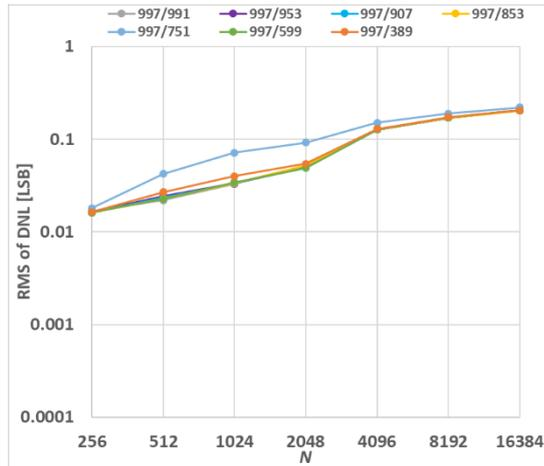
Fig. 4.12 Resolution characteristics of RMS of DNL of prime number ratio samplings by a pair of relatively larger prime numbers (noise 0.1%)
