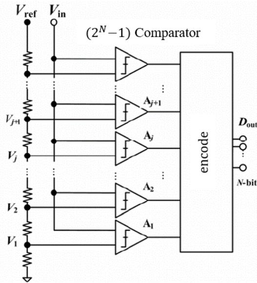
Fig. 2.5 Flash ADC structure.
