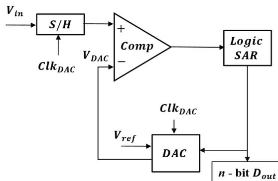
Fig. 2.6 SAR ADC structure block diagram.
