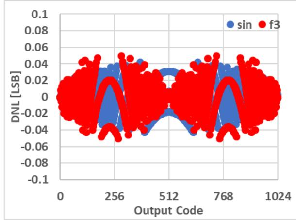
Fig. 3.11 Ideal 10-bit ADC DNL for the input signal of  $f_3(t) = \sin(t) - \frac{\sin(3t)}{3}$  in red and  $f(t) = \sin(t)$  in blue
