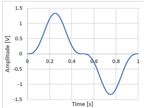
Fig. 3.9 Input wave  $f_3(t) = \sin(t) - \frac{\sin(3t)}{3}$
