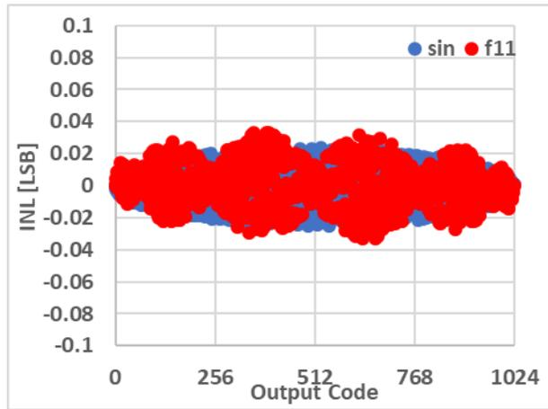
Fig. 3.18 Ideal 10-bit ADC INL for the input signal of  $f_{11}(t) = \sin(t) - \frac{\sin(11t)}{25}$  in red and  $f(t) = \sin(t)$  in blue
