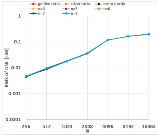
Fig. 4.3 Resolution characteristics of RMS of DNL of metallic ratio samplings
