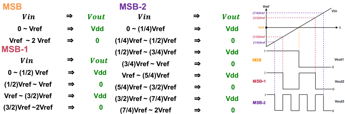
Figure 4.11 Simulation results of the proposed ADC for the ramp input signal (In 3-bit resolution case).
