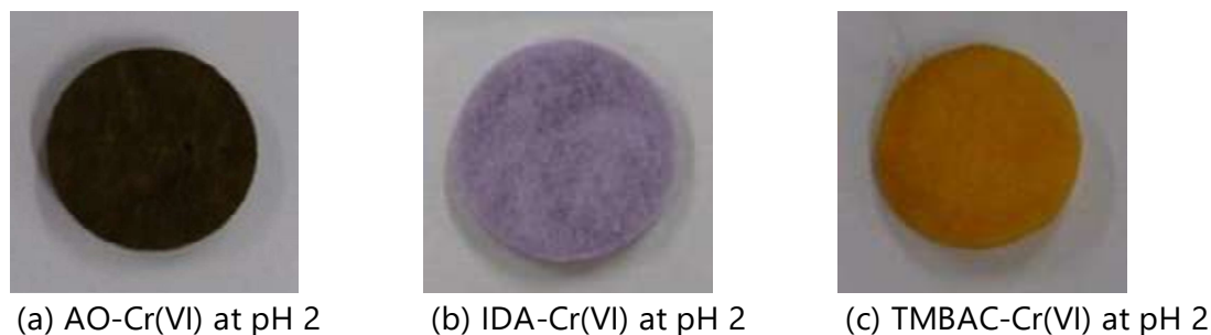
Figure 4-1 Photograph of the adsorbents (a) AO after adsorption of Cr(VI) at pH 2, (b) IDA after adsorption of Cr(VI) at pH 2 and (c) TMBAC after adsorption of Cr(VI) at pH 2.
