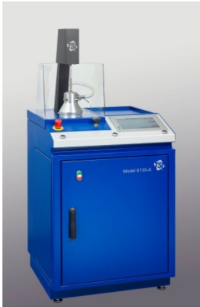
Fig.8 Automated filter tester (AFT8130A, TSI) [37]
