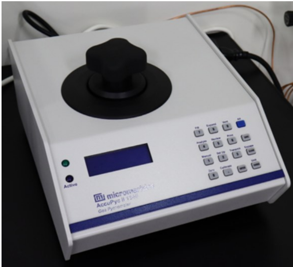
Fig.31 Pycnometer (AccuPyc 1345, SHIMADZU)
