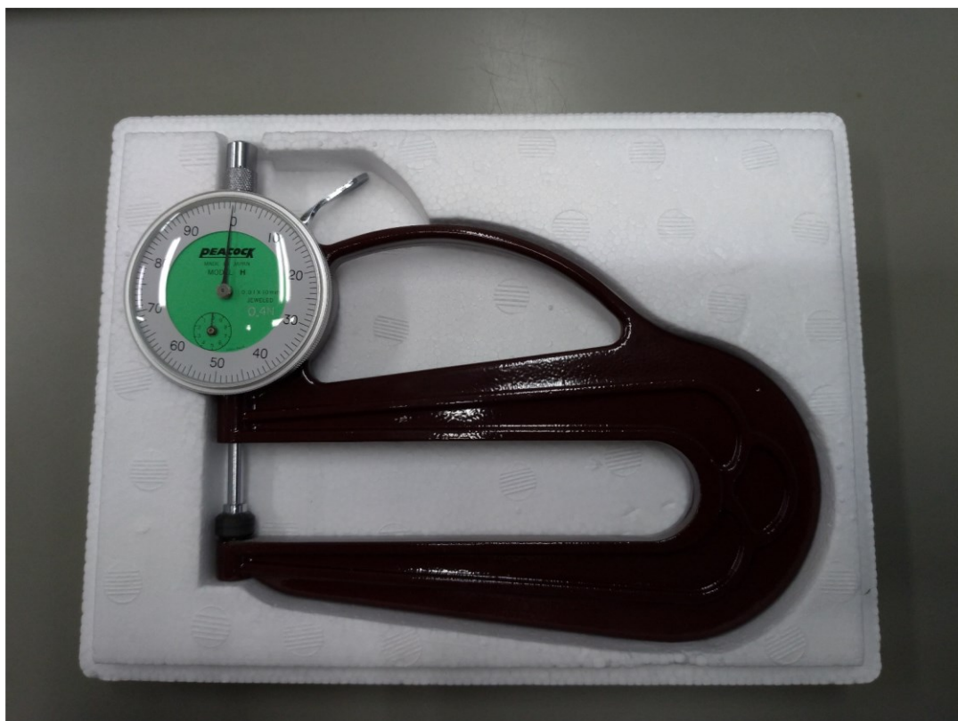
Fig.30 Thickness gauge, (Model H, SHIMADZU)
