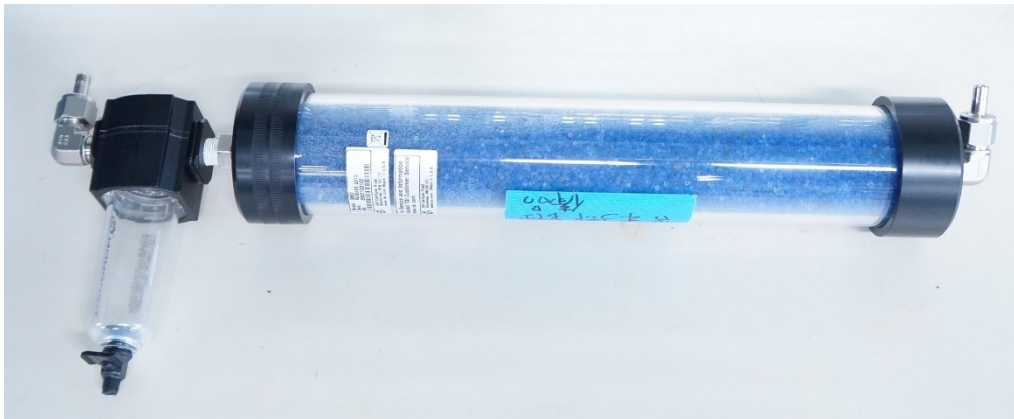
Fig.42 Dryer tube contained within silica
