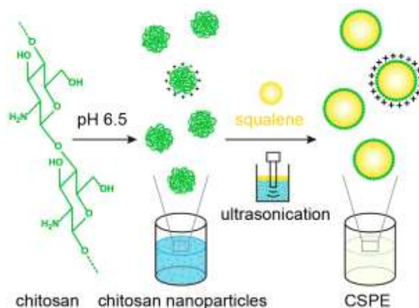
Figure 2.1 Schematic diagram of the preparation process of CSPE
