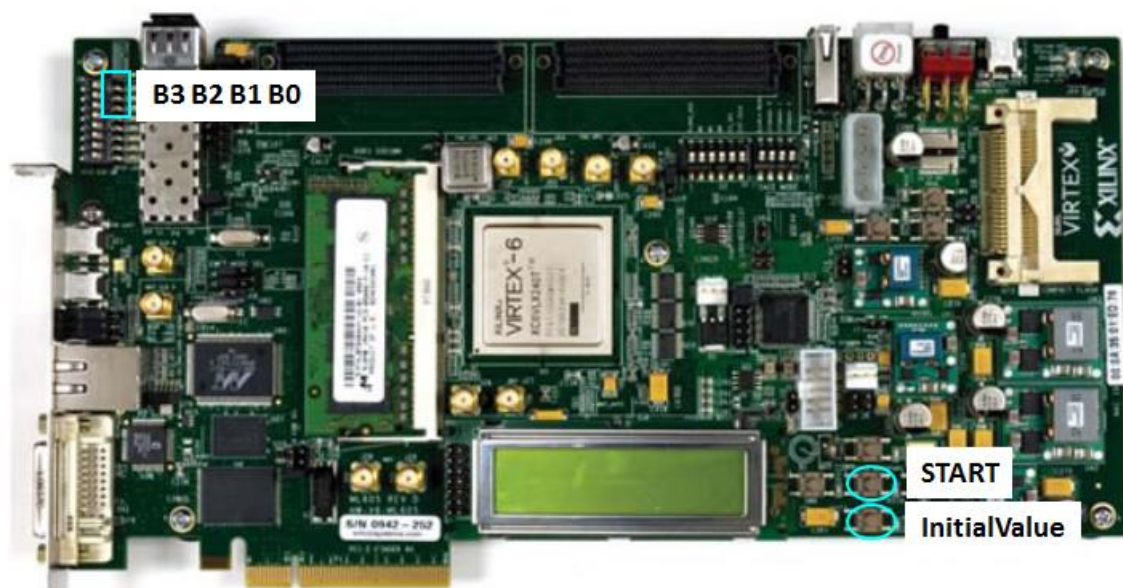
Fig. 3.17 FPGA implementation of 4-bit Gray code TDC
