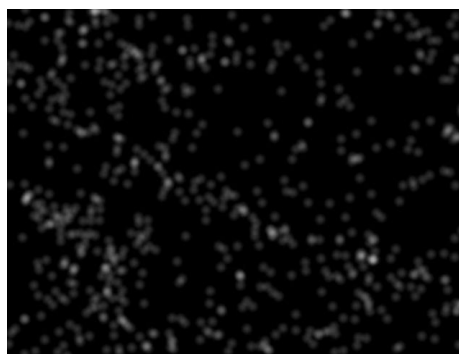
Figure 1.18 Nitrogen elemental map from the EDX analysis of the aminated WHF with 1.78 mmol/gram amino functional group density.
