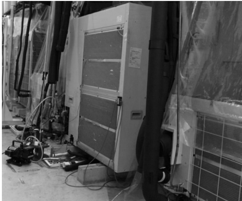
Fig. 2-27 CO 2 - CO 2 binary refrigeration system in test facility of CVS
