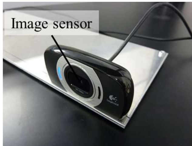
Fig. 2.3 USB camera (HD Webcam C615)
