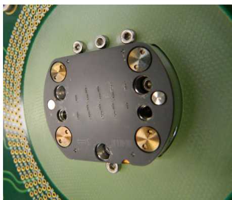
Figure 175 – 16-site EEPROM wafer sort probe head
