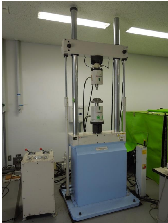
(a) Material tester (Shimadzu EHF-EM100kN/1kNm).
