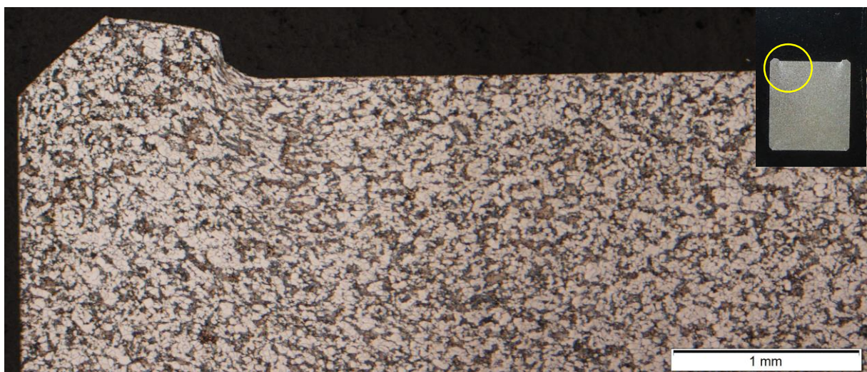
Fig. 2.3-11 Microstructure of corner of cold-forged specimen at CF load of 400 kN.
