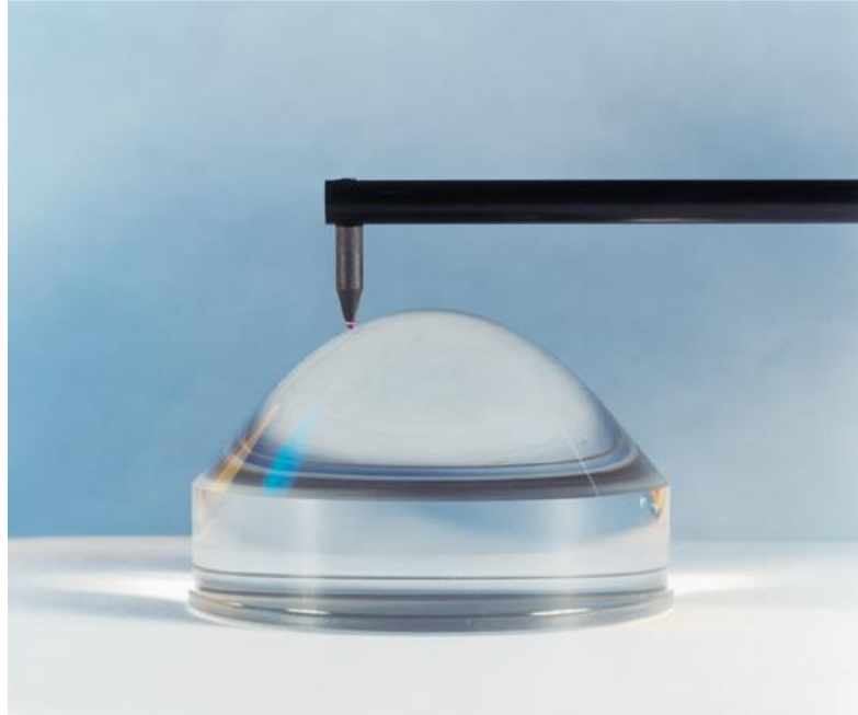
Fig. 1.3 Triggered measurement method by coordinate measuring machine [1]
