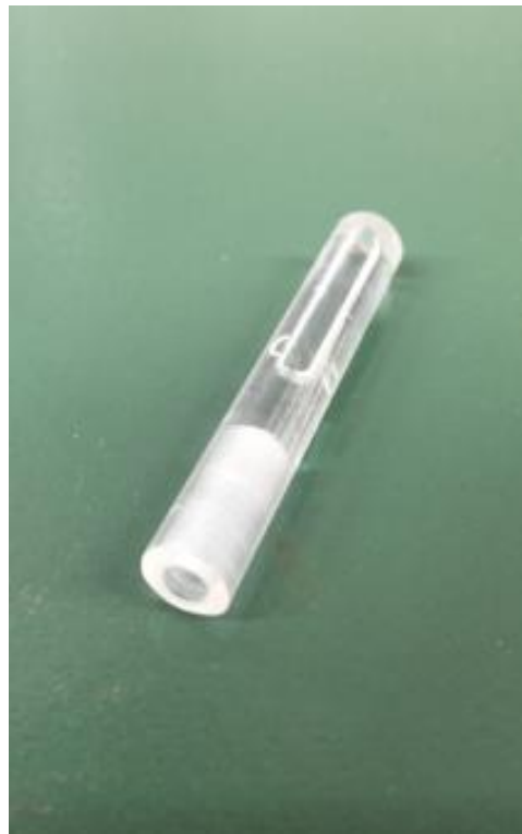
Fig. 2.6 Acrylic polishing tool
