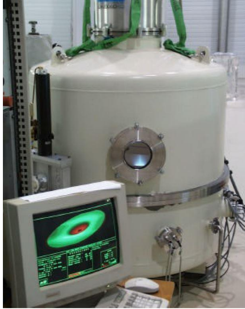
Fig. 1.5 The vacuum chamber of the ion beam facility [21]
