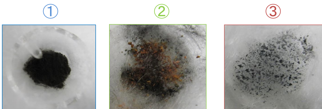
Fig. 4.5 Photos of de-ashed, Cu-loaded Loy Yang brown coal (Cu-loading:8.56wt%) during burning in a simulated air atmosphere ① before heating, ② at 165°C and ③ at 180°C
