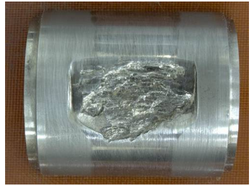
(f)複合 CD 浸炭, \text{NH}_3 0.50 \text{m}^3/\text{h}
