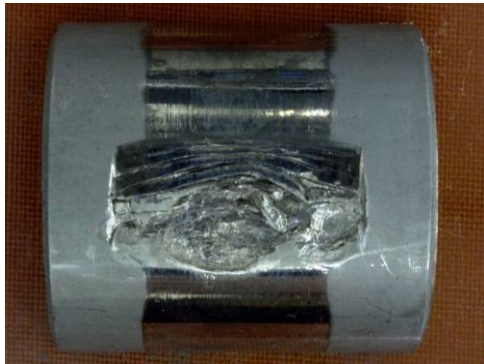
(e)複合 CD 浸炭, \text{NH}_3 0.35 \text{m}^3/\text{h}
