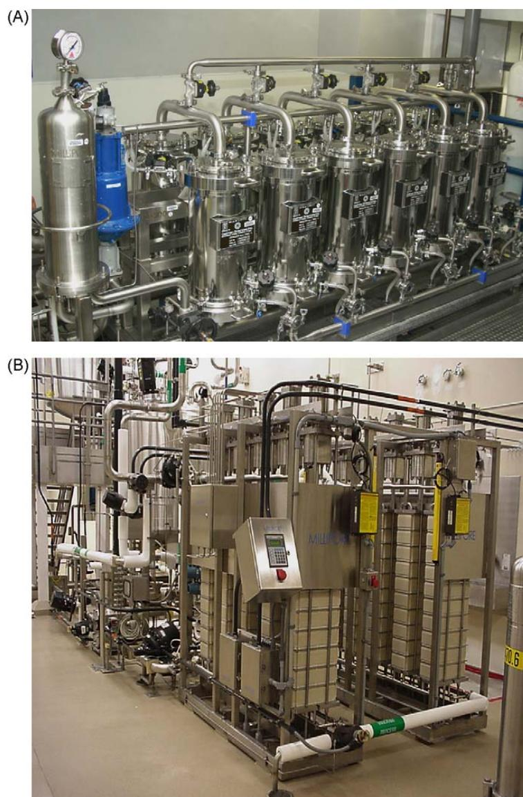
Fig. 1.4. (A) Microdyn 0.2 µm polypropylene hollow fiber microfiltration system with 174 m<sup>2</sup> membrane area. (B) Millipore Prostack™ flat sheet membrane system with 186 m<sup>2</sup> of 0.65 µm pore size hydrophilic PVDF membrane [7].
