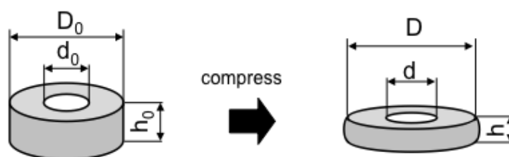
Fig 2.3 Deformation of ring specimen during compression
