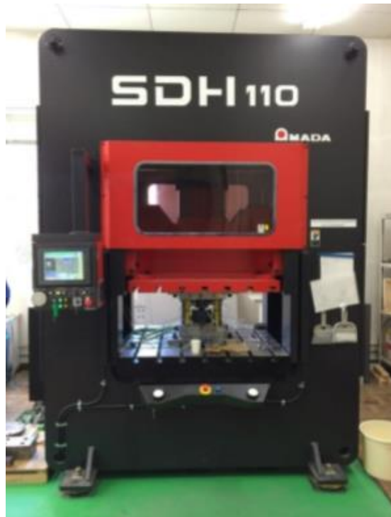
Fig 3.1 Photos of the appearance of forging press
