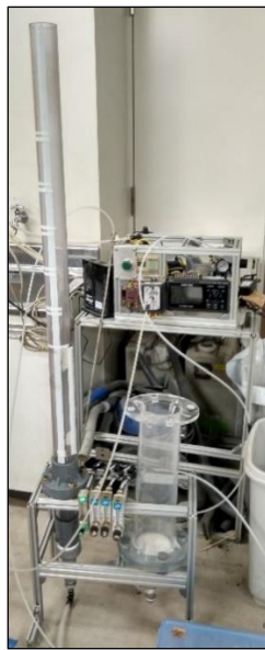
Figure 2-3. Bubble system for elutriation process
