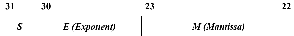
Fig. 7.2 IEEE-754 floating-point format (single precision case).
