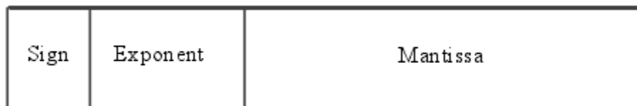
Fig. 2.1 Format of floating-point number
